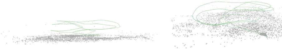
**Fig. 7.** Side-view of the generated sparse point-cloud and the estimated trajectory flown by the UAV. The right figure shows take-off and landing spot with increased point-cloud density.
